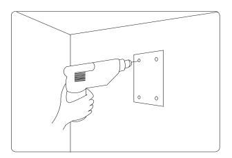
Fasten the wall bracket by plugs, taking care to leave the cable outlet at the center between the fixing holes.
