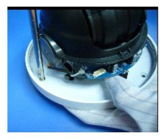
Screw the collar to complete the installation
