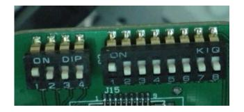
The microswitch 4 block is used to set the baud rate.
